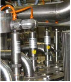
HYDROSTATIC LEVEL MEASUREMENT
